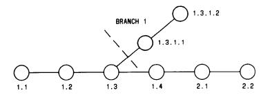
Figure 8.2. Tree Structure With Branch Deltas
