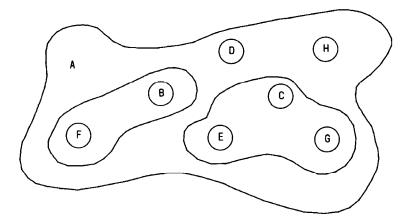
Figure 9.3. UUCP Network With Several Levels of Permissions
